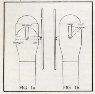
5. Move the throttle or "fuel" lever (Fig. 1b) forward to approximately the half speed position.
